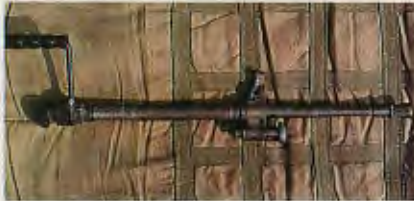
ABOVE: Handled barrel assembly helps hot-barrel change. RIGHT: Operator's eye view of open SAW feed cover. BELOW: M249 spits links in full-auto fire.
